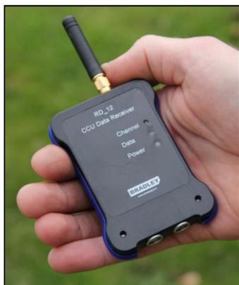
An **RD\_11** Data Transmitter can transmit to multiple **RD\_12** CCU Receivers for radio CCU control.
