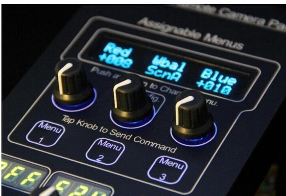
The Assignable Menu sets this RCP apart from others. To minimise the number of knobs and buttons and maximise the information display area, a user assignable menu is used for less often needed parameters. There are 3 instantly accessible menus, each with 3 adjustable parameters.
