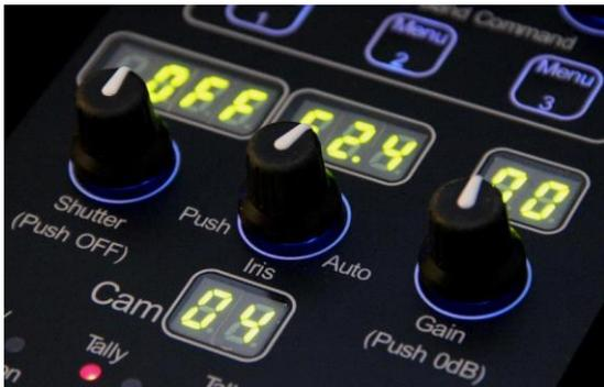
Clear LED readouts display the major settings for each camera as it is selected; Iris, Gain, Shutter, Camera No. etc.
