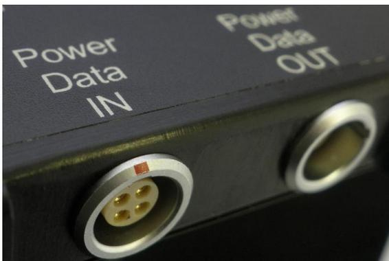
Industry standard Lemo sockets are used for both inputs and outputs. Power is looped through with various output options available on the 7 pin output socket.
