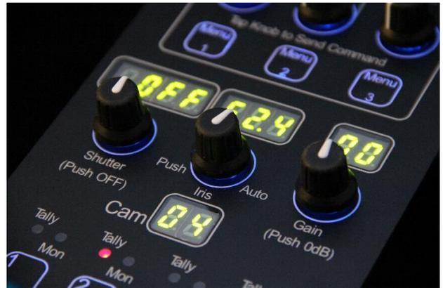
On the latest models, a brief touch down on the '**Iris**' knob toggles control of the **Iris** or **ND Filter** from the Iris Joystick. Iris can always be controlled with the centre knob. Push and hold on the '**Iris**' knob switches the camera to **Auto Iris** (if supported). The Iris display will show if BARS are selected.
