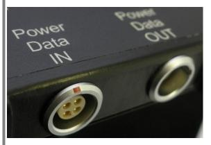
Industry standard Lemo sockets are used for both inputs and outputs. Power is looped through with various output options available on the 7 pin output socket.
