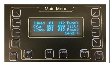
When ALL the numbers are correct push the '**Send**' button at the bottom right. This will send all the values to the remote head.
