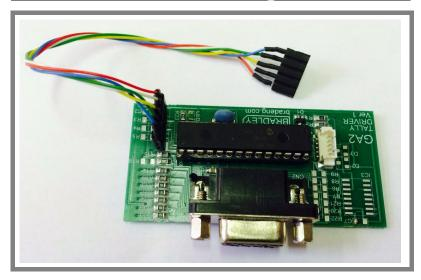
Fitting the Monitor Switching Module is very simple but the connectors **MUST** be orientated as shown in the pictures. Once installed, check carefully the wiring colors match the pictures **before** powering the unit up.
