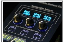
To assign a different parameter to a knob simply push down on the knob and rotate it to change the function. When the knob is released the knob now controls the parameter shown. If the function requires a switch action a brief touch down on the knob toggles the switch action.
