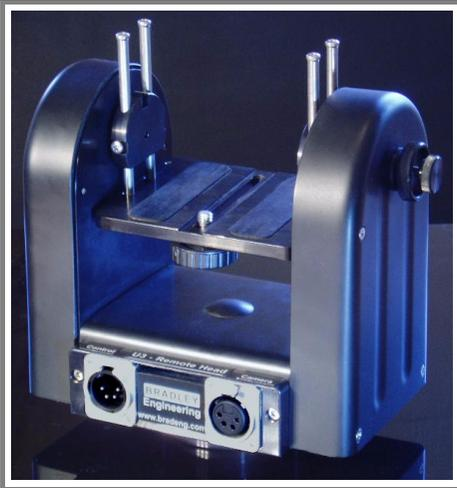
The **U3/S Remote Head** is a small but fully featured pan & tilt head which offers both live action moves, preset positions, and full camera and lens control using RS485 data. The head is weatherproof and can be used externally without further protection.
